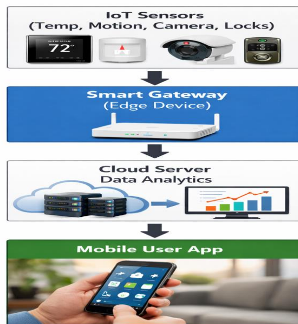
Figure 1: Typical Smart Home Communication Architecture
